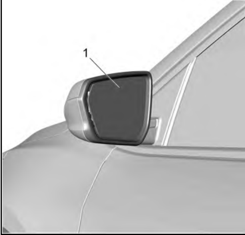
Outside Rearview Mirror Glass (1) - Remove - Outside Rearview Mirror Glass Replacement
