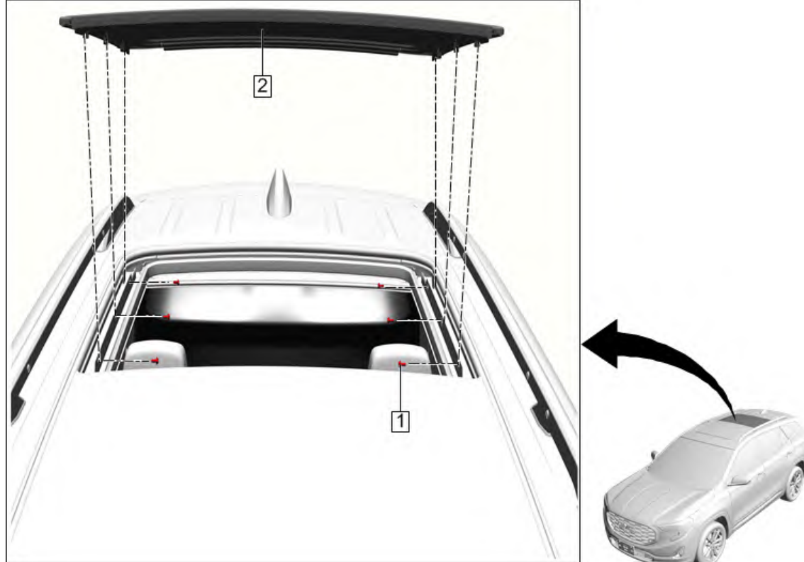
Fig. 41: Roof Stationary Window (Terrain). Courtesy of GENERAL MOTORS COMPANY
