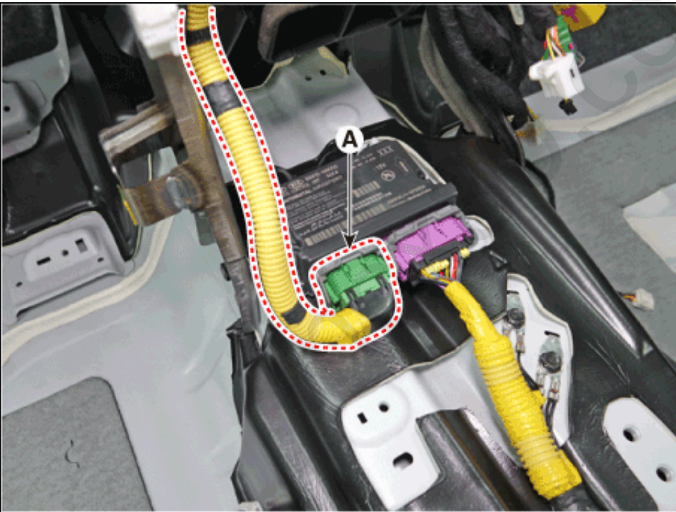
24. Disconnect the passenger compartment junction box connectors (A).
